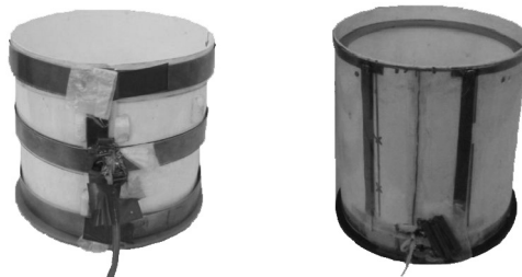
Fig. 1. Sensor "joint" of the cylindrical type, the receiving system to the left, to the right of the transmission system.
